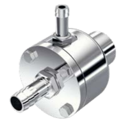
DK 25.11 Flow chamber For S 25 KV - 25 ... - IL dispersing elements. Batch operation: DK 25.11 is mounted around the dispersing element. The DK 25.11 must be at a lower elevation than the surface of the liquid during operation. With this operating mode, no air is drawn in as a result of turbulence in the vessel.
