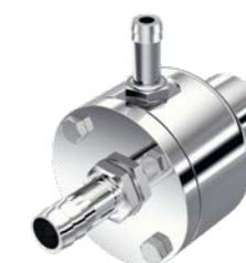
DK 25.11 Flow chamber For S 25 KV - 25 ... - IL dispersing elements. Batch operation: DK 25.11 is mounted around the dispersing element. The DK 25.11 must be at a lower elevation than the surface of the liquid during operation. With this operating mode, no air is drawn in as a result of turbulence in the vessel.
