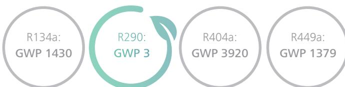
This means a reduction of the global warming potential to only 0.21% on the base value of R134a. This does not yet take into account that the refrigerant charge quantities for R290 can also be reduced.
